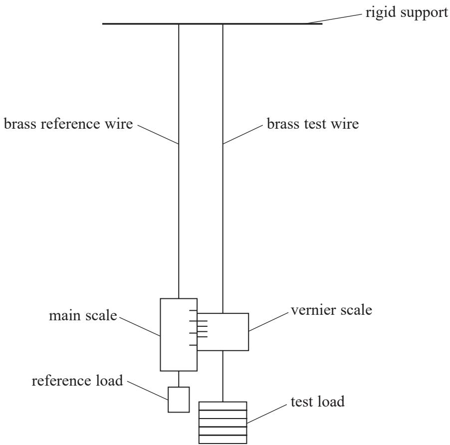
(a) (i) Give one advantage of using a reference wire as well as a test wire.
